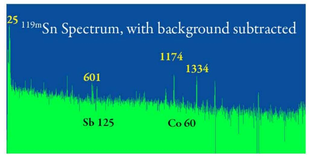
The background-subtracted sample has fewer peaks, and allows us to more easily identify the impurities in the sample. The main impurities were <sup>60</sup>Co, <sup>75</sup>Se, <sup>113</sup>Sn, <sup>125</sup>Sb, and <sup>182</sup>Ta.
